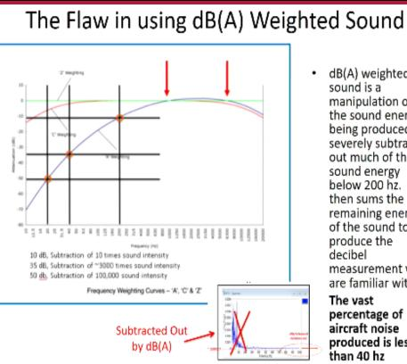
dB(A) weighted sound is a manipulation of the sound energy being produced. It severely subtracts out much of the sound energy below 200 hz. It then sums the remaining energy of the sound to produce the decibel measurement we are familiar with The vast percentage of aircraft noise produced is less than 40 hz
