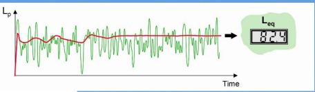
$L_{Aeq(T)}$  is the equivalent continuous A-weighted sound pressure level (dB(A)) measured over the time period T;
